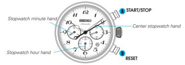
Current time indication: 10 o'clock 8 minutes and 42 seconds Stopwatch time indication: 6 hours 20 minutes and 10 seconds
