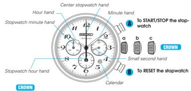
a) Normal position : winding up the mainspring (manual operation)
