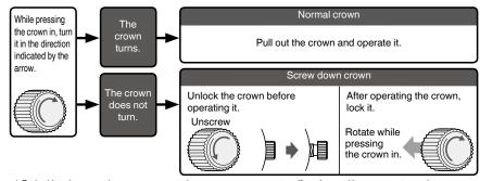
\* By locking the crown by screw, a screw down crown can prevent malfunction and increase water resistance.
