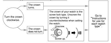
After completing all settings of the watch, screw the crown up again by turning it clockwise while pressing it.
