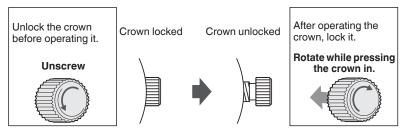
\* When locking the crown, turn it slowly with care, ensuring that the screw is properly engaged. Be careful not to push it in forcefully, as doing so may damage the screw hole in the case.
