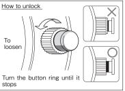
Turn the button ring counterclockwise (6 o'clock Turn the button ring clockwise direction) to lower the slide cover gradually. Turn (12 o'clock direction) until it the button ring further until you can clearly see stops. Now the screw-lock the guide line and the button ring can no longer type button is completely be turned. Now the screw-lock type button is locked. Once you have unlocked and can be operated.
