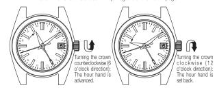
Turn the crown slowly, checking that the hour hand moves in one-hour increments. While turning the crown, the moment the date changes is midnight. When setting the hour hand, the other hands may move slightly. However, this is not a malfunction.
