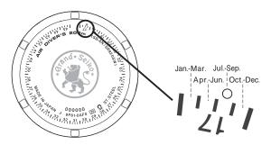
Arabic numerals on the scale show the last two digits of the year. For subsequent battery replacements, a circle mark will be engraved each time a watch is returned to an authorized Grand Seiko retailer for battery replacement or watch repair.
